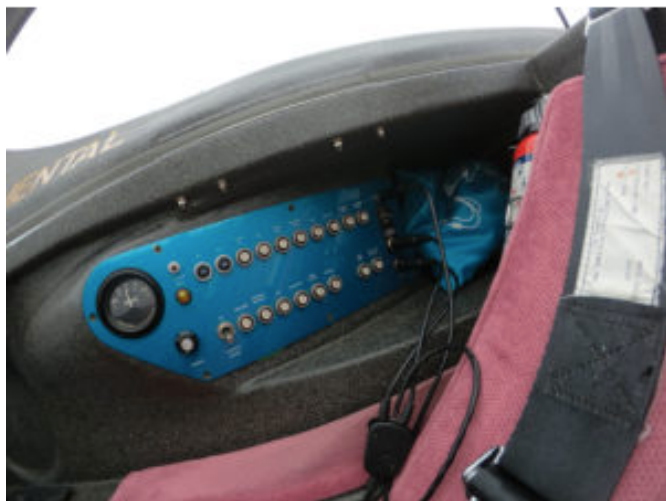
Strake mounting the electrical panel is handy and frees up instrument panel space.
