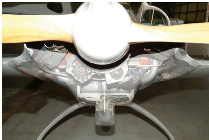
Terry Schubert's Long-EZ engine installation is artfully revealed in this double-exposure shot, taken before and after the cowling was installed.
