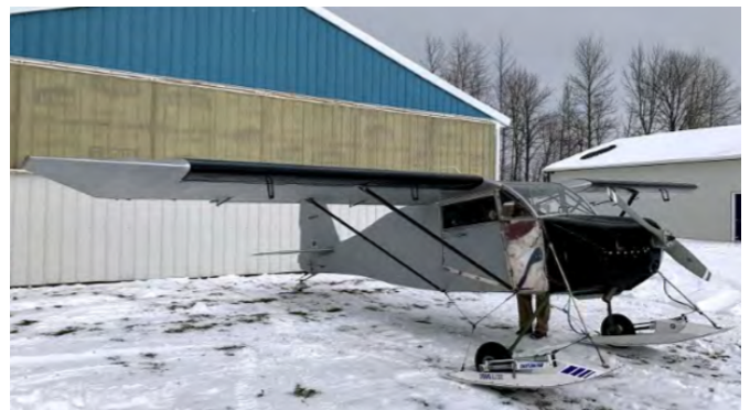
Jeff LaChausse's 150 hp Buttercup with Datum retractable wheel ski's
